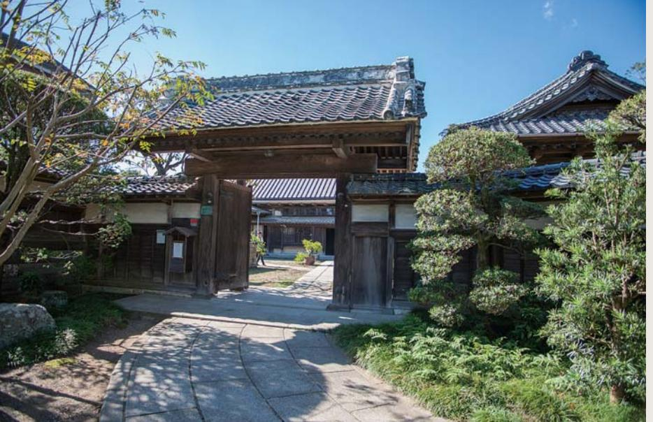
The front gate is a full-fledged yakui-mon gate constructed in the end of the Edo Period. These are characterized by having two main pillars and two support pillars in the rear that undergird a gabled roof.
